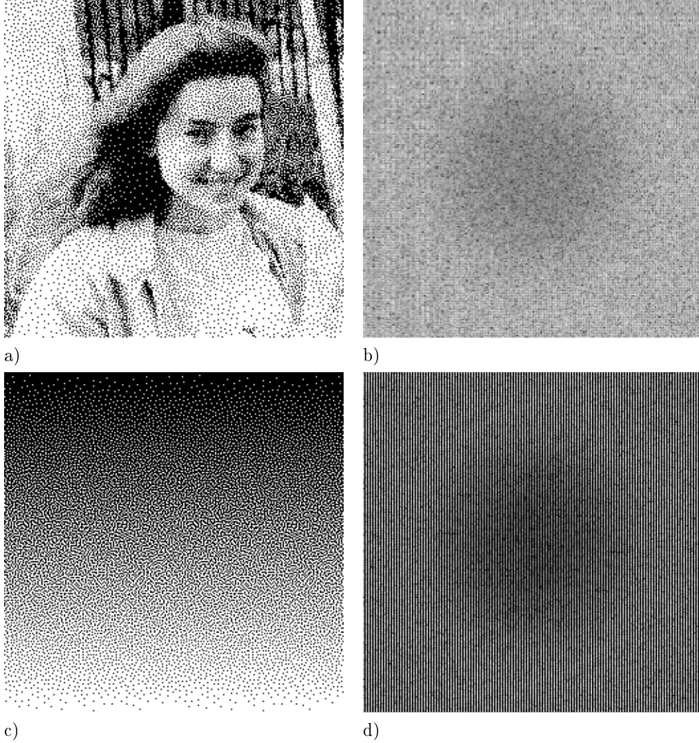
Fig. 4. Ordered dither with a blue noise mask (void-and-cluster): Halftone representations of test images (left); the magnitude spectra of the corresponding noise images (right). a) Portrait of Anya Pogoyants b) Magnitude spectrum of the noise image (min = 0.14, max = 6.2) c) Gray scale ramp d) Magnitude spectrum of the noise image (min = 0, max = 6.4)
